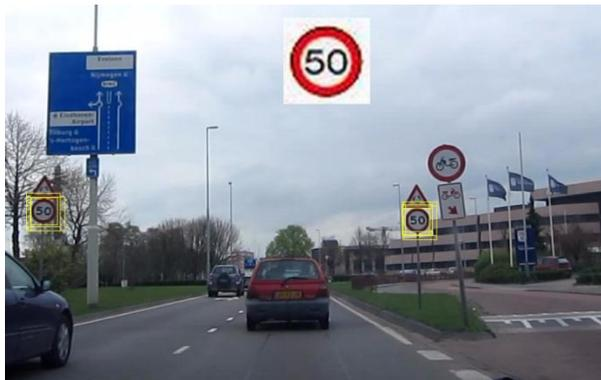
Fig. 7 Detector output for a 50 km/h speed sign
