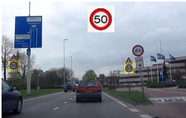
Fig. 7 Detector output for a 50 km/h speed sign
