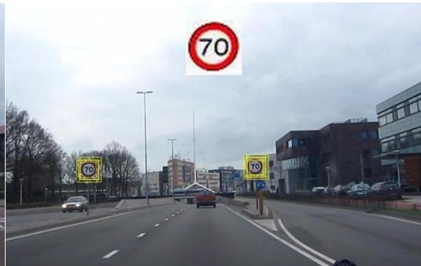
Fig. 8 Detector output for a 70 km/h speed sign
